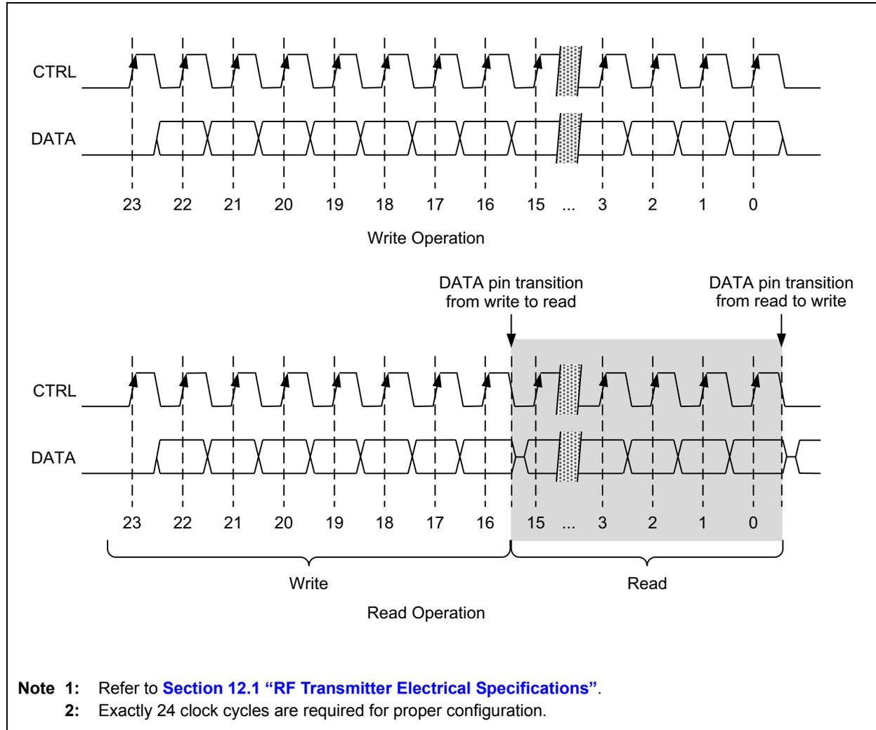
**FIGURE 9-4: RECOVERY SEQUENCE TIMING**
