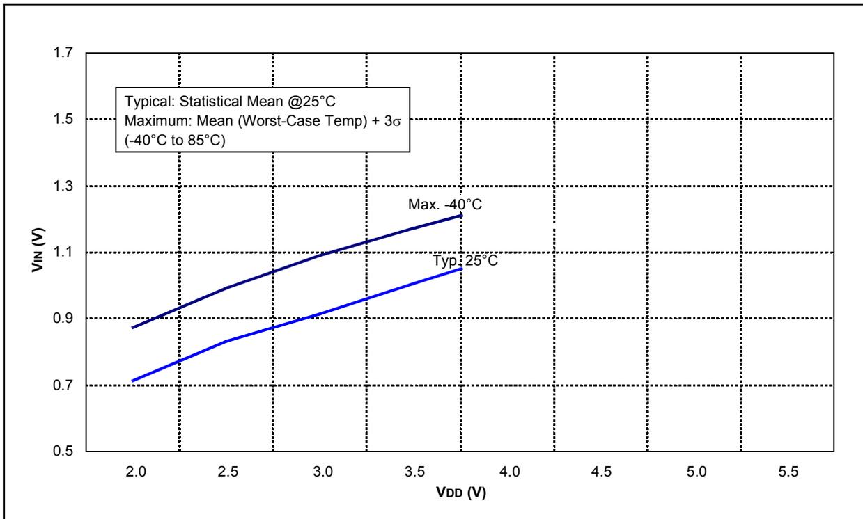
**FIGURE 13-12: SCHMITT TRIGGER INPUT THRESHOLD  $V_{IN}$  vs.  $V_{DD}$**
