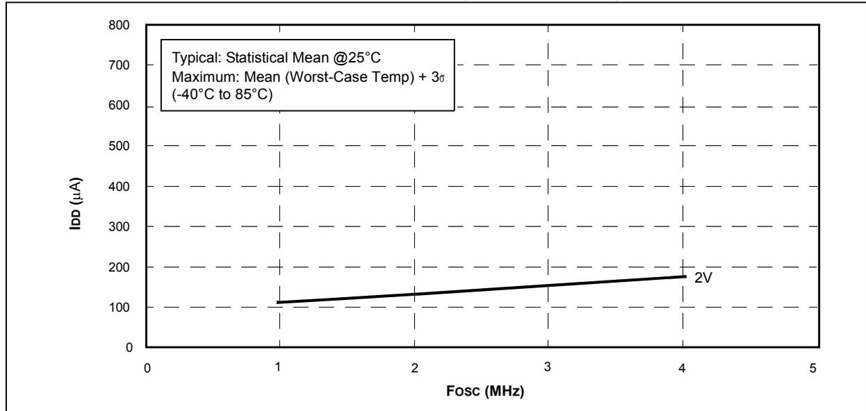
**FIGURE 13-2: MAXIMUM  $I_{DD}$  vs. Fosc OVER  $V_{DD}$  (XT, EXTRC mode)**
