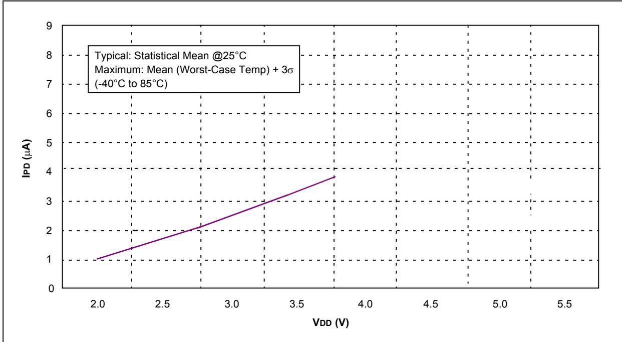
FIGURE 13-7: MAXIMUM WDT IPD vs. VDD OVER TEMPERATURE
