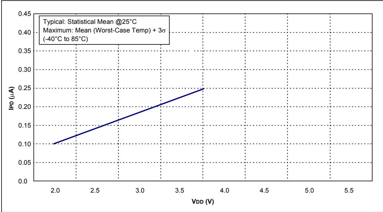
**FIGURE 13-5: MAXIMUM  $I_{PD}$  vs.  $V_{DD}$  (SLEEP MODE, ALL PERIPHERALS DISABLED)**
