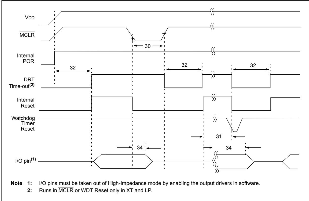
**TABLE 12-8: RESET, WATCHDOG TIMER AND DEVICE RESET TIMER – PIC12F529T39A**
