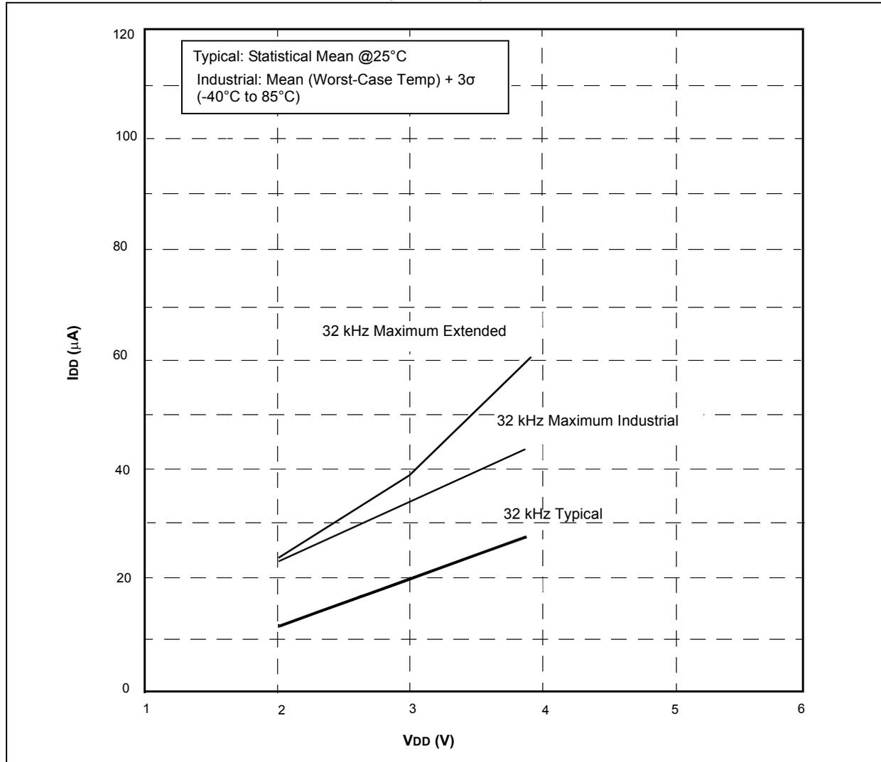
**FIGURE 13-4: TYPICAL  $I_{PD}$  vs.  $V_{DD}$  (SLEEP MODE, ALL PERIPHERALS DISABLED)**
